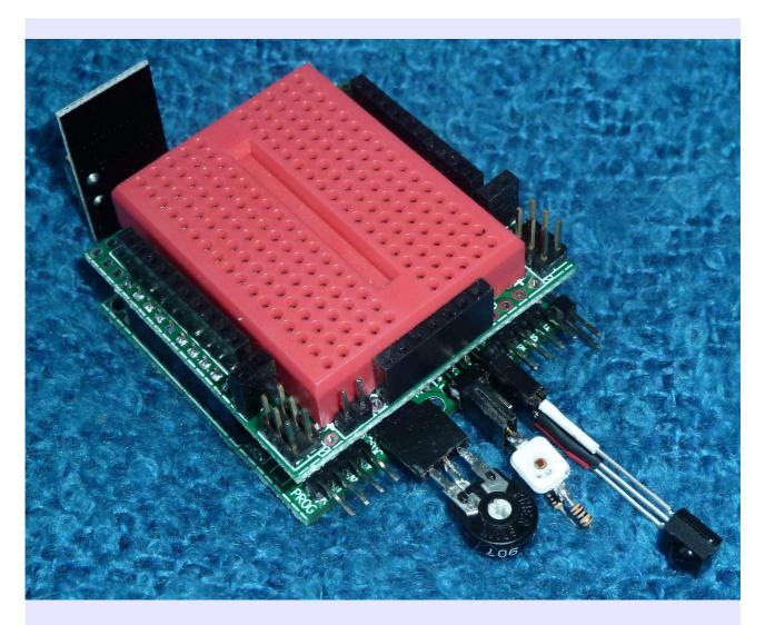
Egel shield top side finished and mounted on the Egel kit
