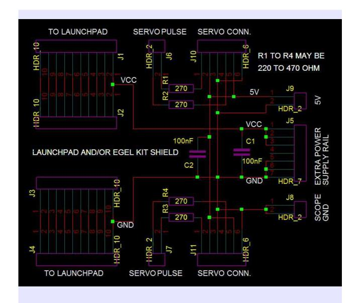
Schematic for Lanchpad/Egel kit shield
