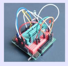
Egel shield wired as cloning programmer
